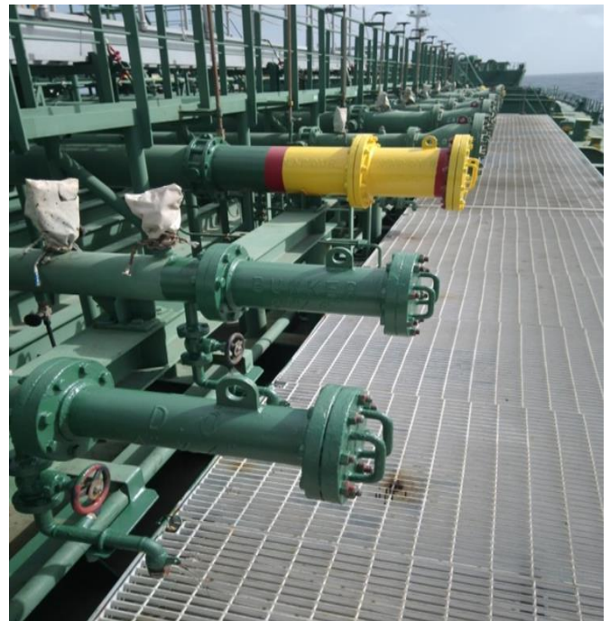
Fig. 7. Properly maintained manifolds on deck through which the cargo loading is done.
