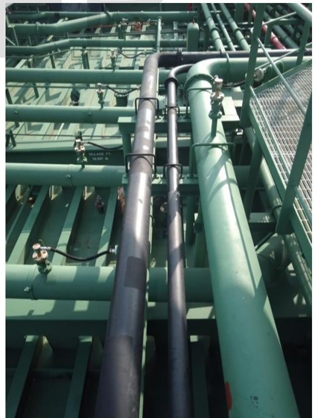
Fig. 8. A way of pipes on deck in order to prevent cracking and stretching due to sagging and hogging.
