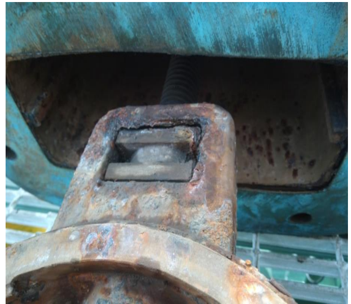
Fig. 5. General corrosion associated with a valve on a fire pump on the upper deck of the ship.
